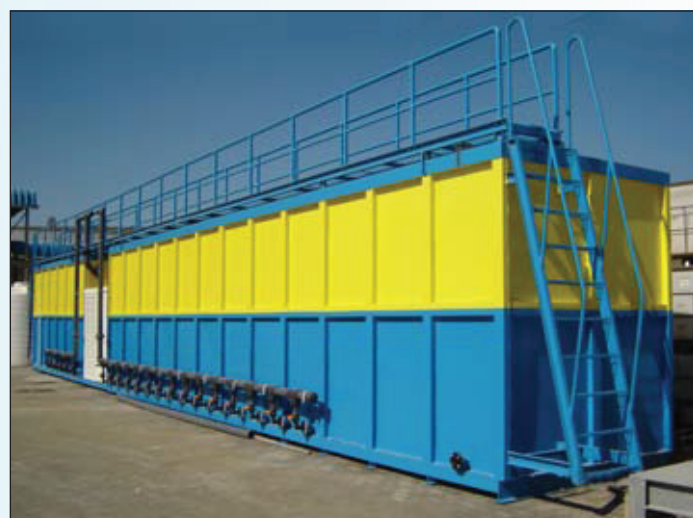
EfloSAF for Ministry of Public Works Kuwait. 300 m 3 /d. TSE < 10 mg/l BOD, SS < 10 mg/l, HN 3 -N < 5 mg/l
